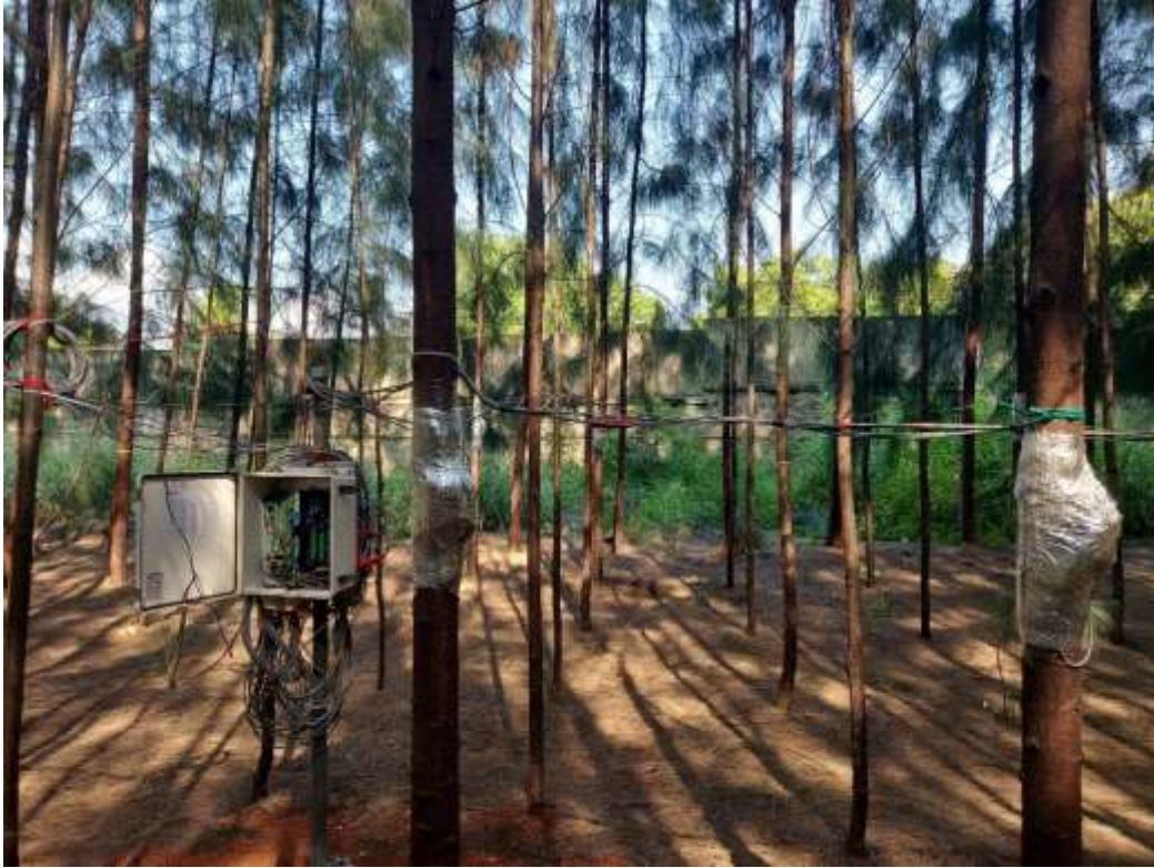
Fig. 2. Recording of water use by selected Casuarina clones using Sap Flow Meter
