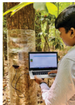
Fig. 16 Data acquisition from sap flow meter
