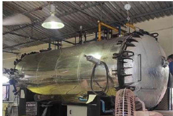
Fig. 8 RF Vacuum Dryer
