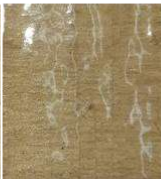
Fig. 10 Coated with PVA/ 0.7%E/ 3%CNC
