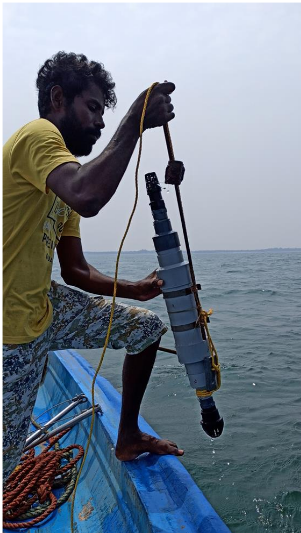
Figure 3.6: (Bottom left) Deployment of Water sampler to collect water samples from seagrass meadows
