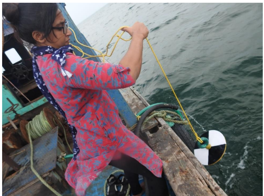
Figure 3.3: Water clarity determination using Sechchi Disc
