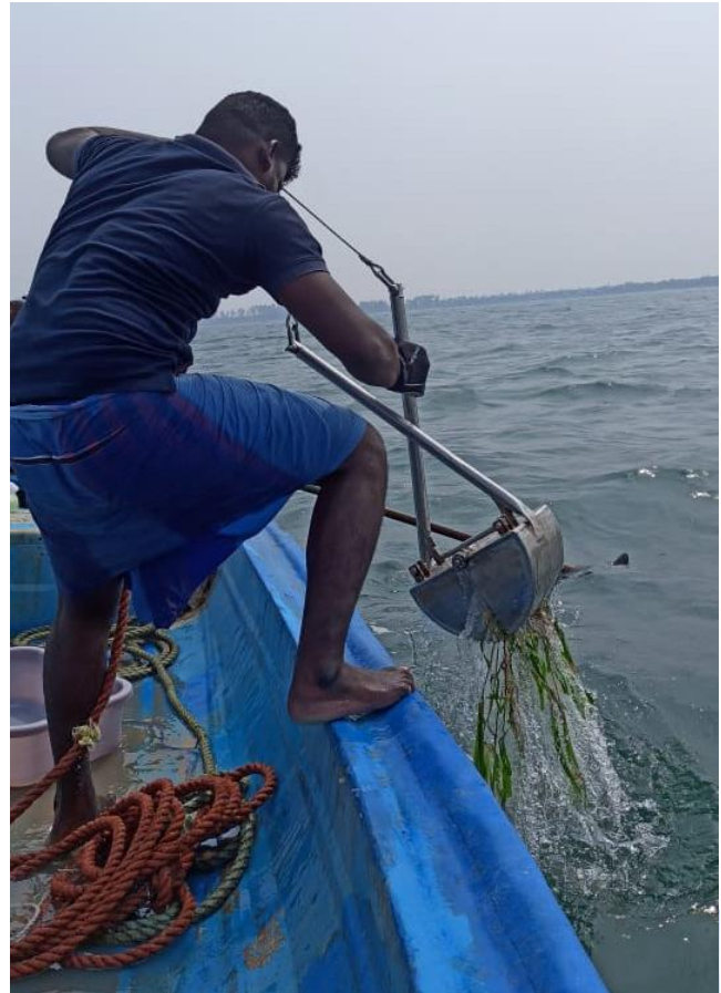
Figure 3.6: (Bottom left) Deployment of Water sampler to collect water samples from seagrass meadows
