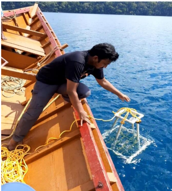
Figure 4.13: Quadrat with attached camera used for survey to check presence-absence of seagrass (in left), environmental parameters recording dugong seagrass survey (in right)
