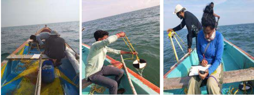
Figure 35. Structure for drop down quadrat with GoPRO fixed on it. B. Assessing the transparency using a Secchi Disk. C. Dropping of the quadrat
