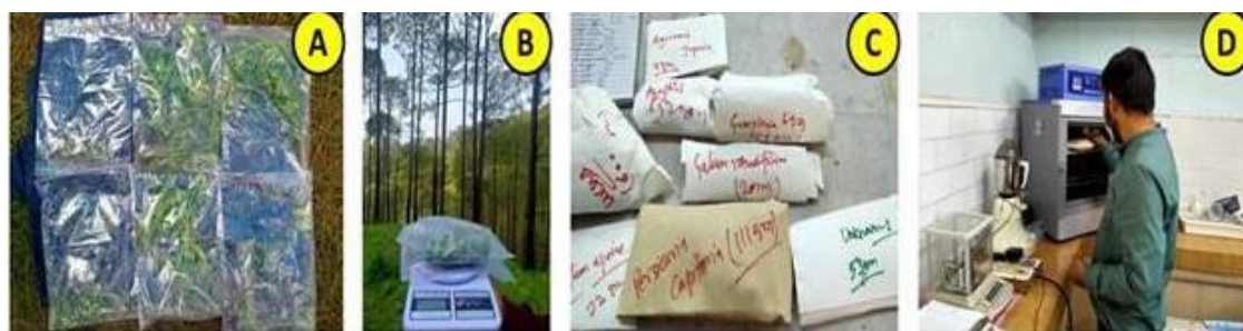
Fig. 1 Step-wise method for biomass estimation of the useful/tradable part of the species (A) categorization of bushes of different size; (B) measurement of fresh weight of the useful/tradable part at the field; (C) preparing species for oven dry (D) oven dry of species at lab
