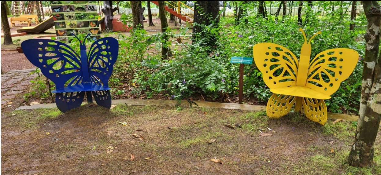
Design, profile cutting fabrication, fitting welding and assembly, primer coating and painting (03 Coats) of Butterfly shaped butterfly design kids chair for Butterfly Park at Bio Diversity Park, Mollem
