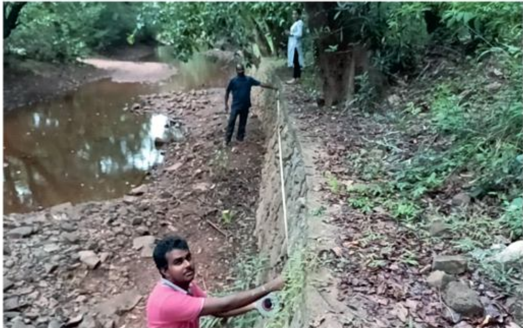
Gully plug dimension assessment
