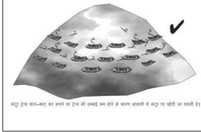
Staggered contour trenching
