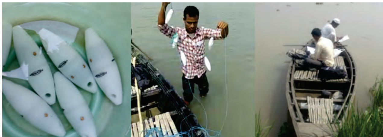
Pingers are small acoustic deterrents that emit sonic pings to help dolphins detect the presence of the net, and thereby reduce their chances of entanglement. Their deployment is depicted here.
