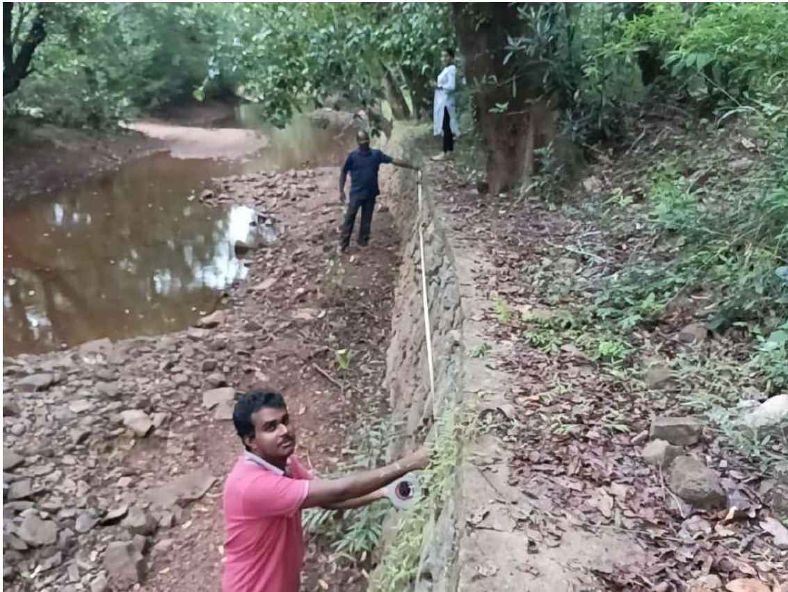
Gully plug dimension assessment
