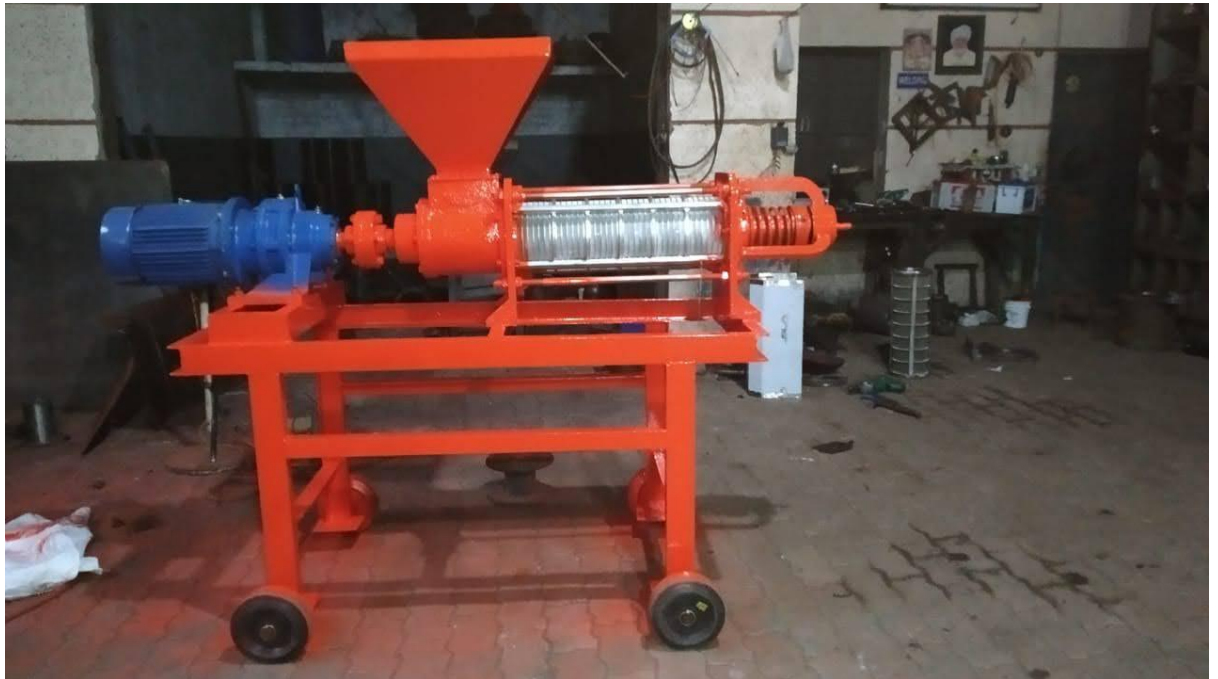
Dewatering Machine reduces water from 85% to 15% to make drying faster
