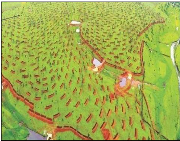
Fig 3.6: Staggered Trenches (SGT)
