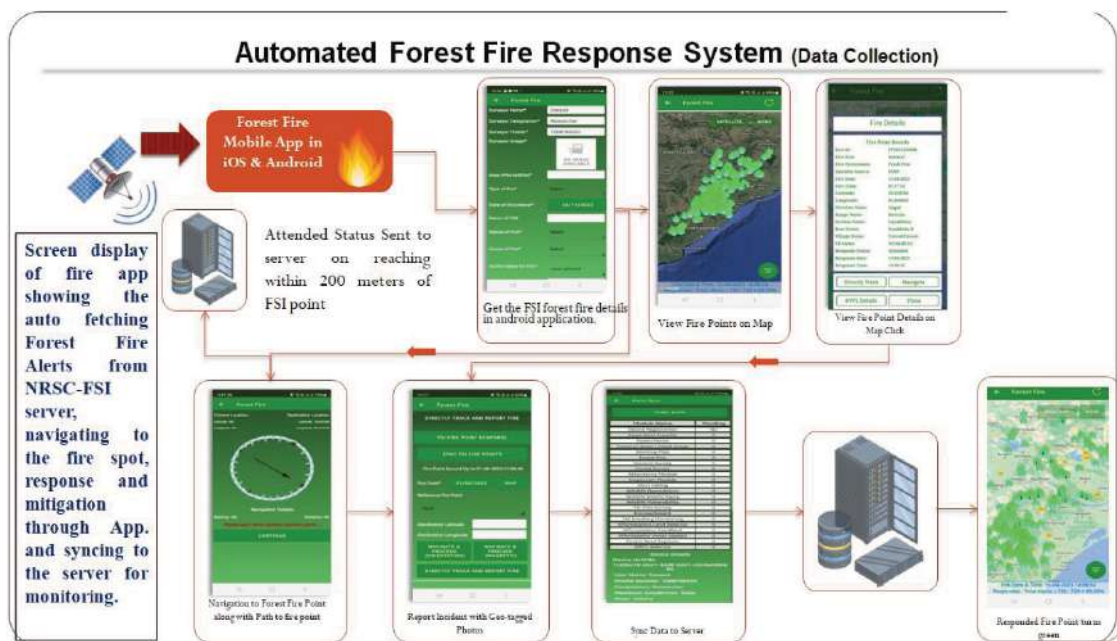
(Screen display of fire app showing the auto fetching fire points from FSI server, navigating to the fire spot, responding through App. and syncing to the server for monitoring.)
